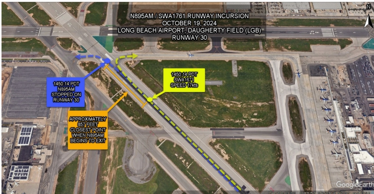
Figure 1. Overhead view of the flight tracks of N895AM and SWA1671 with the area of closest proximity.
