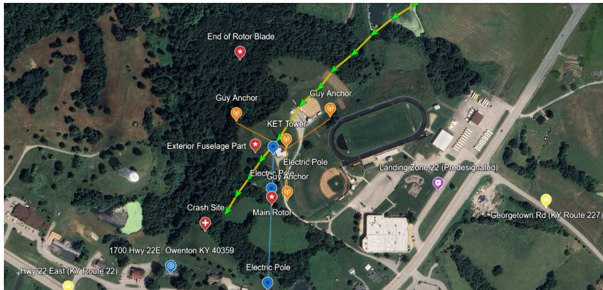
Figure 1 - Aerial image with the helicopter's ground track, as well as positions of the accident site, select pieces of wreckage, the tower and guy anchors, and the LZ annotated.
