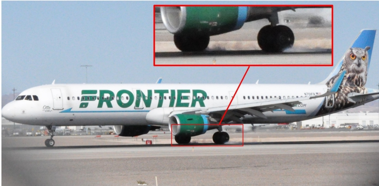
Figure 2. Photograph showing smoke trailing behind N701FR's main landing gear (Source: Owen Denning).
