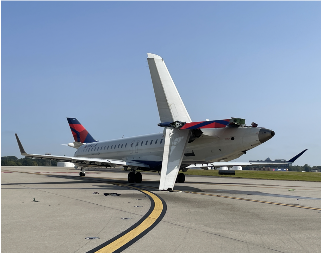
Figure 1. Photograph showing the CRJ after impact. (Source: Atlanta Airside Operations)
