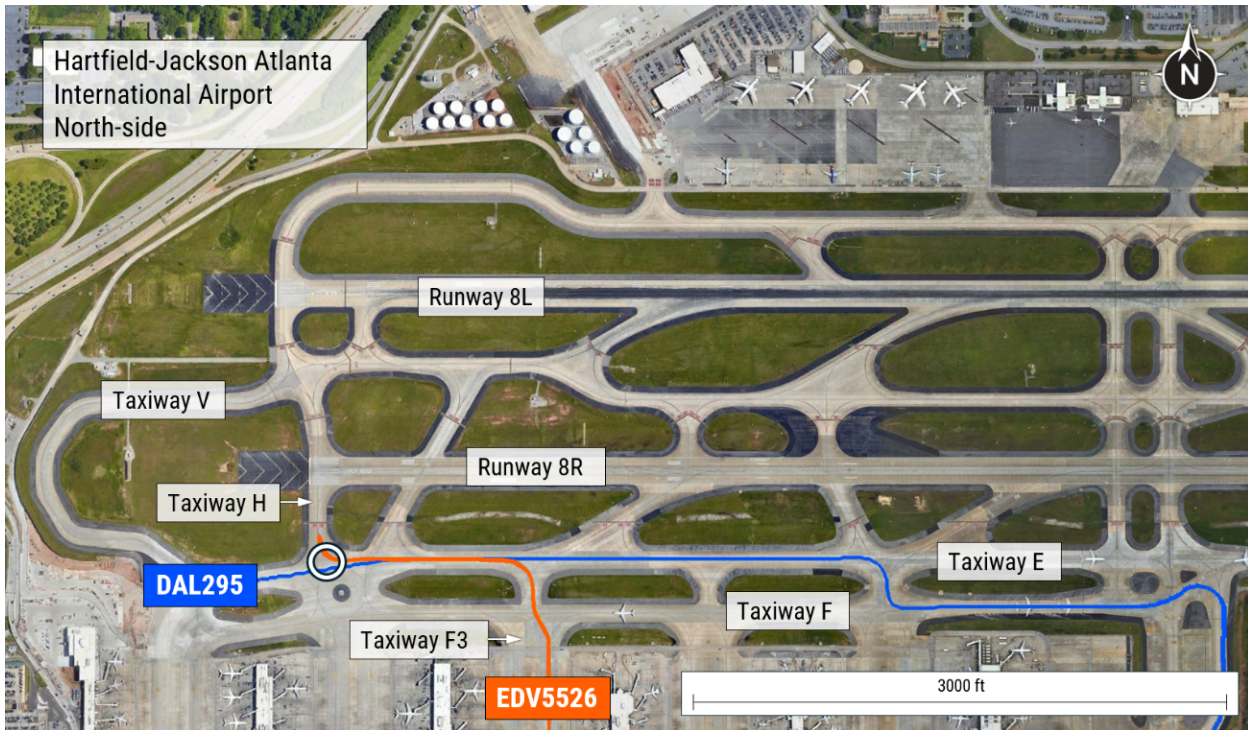
Figure 2. Ground position tracks for DAL295 (A350) and EDV5526 (CRJ) in relation to taxiways E and H.
