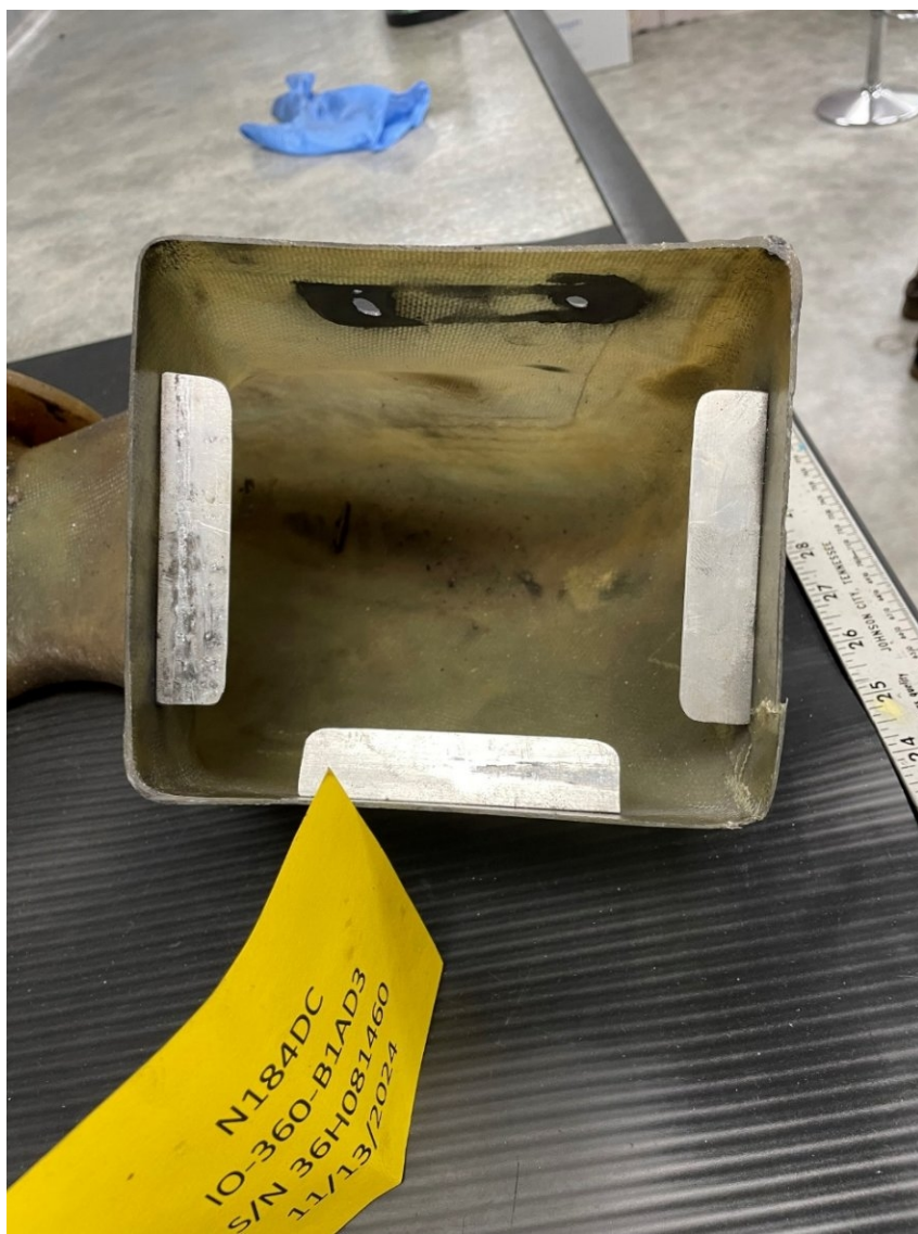
Figure 1. Air filter retaining brackets; one bracket separated and missing.
