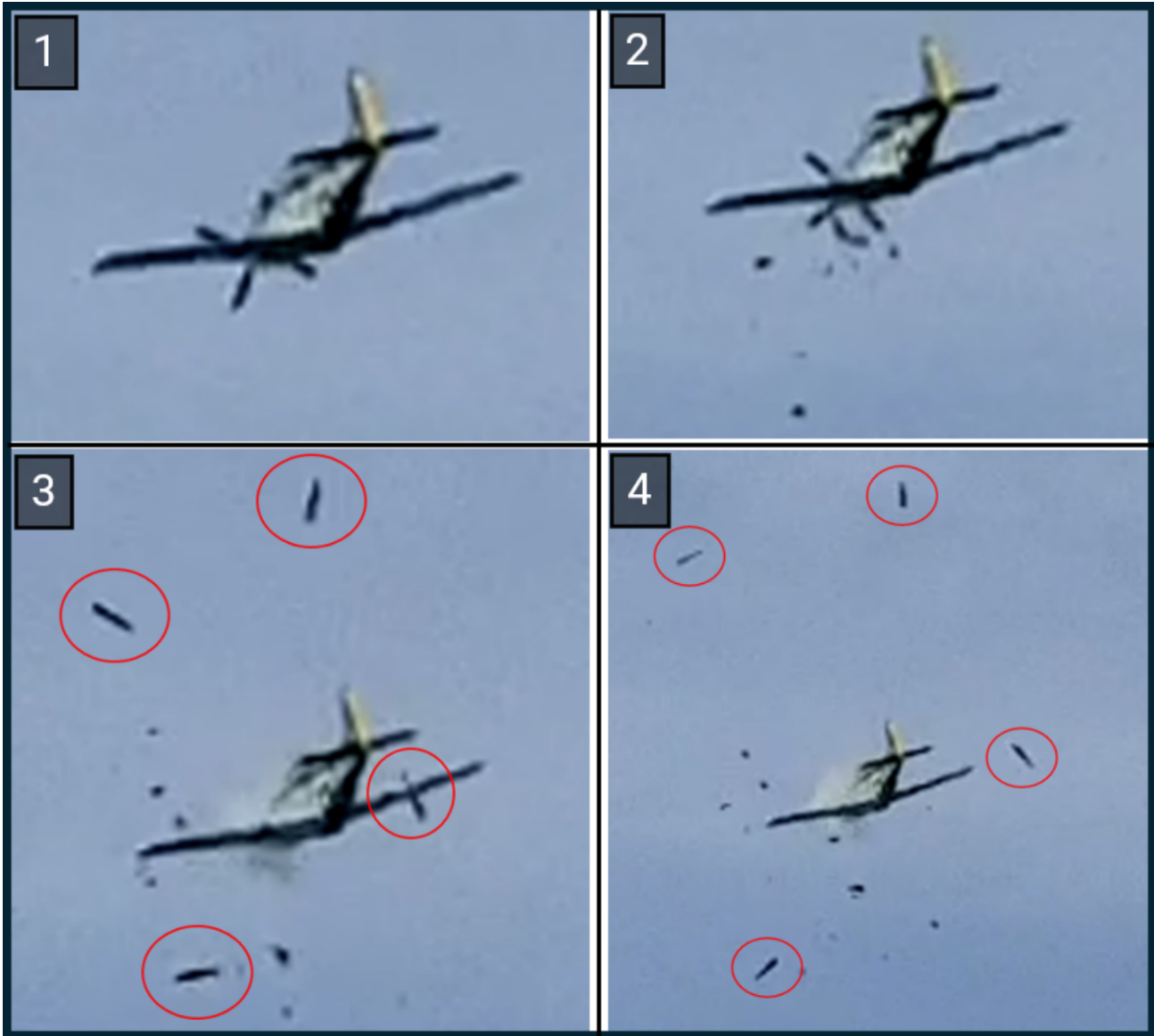
Figure 1: Frame by frame view of the parts separation (the red circles outline the four propellers).
