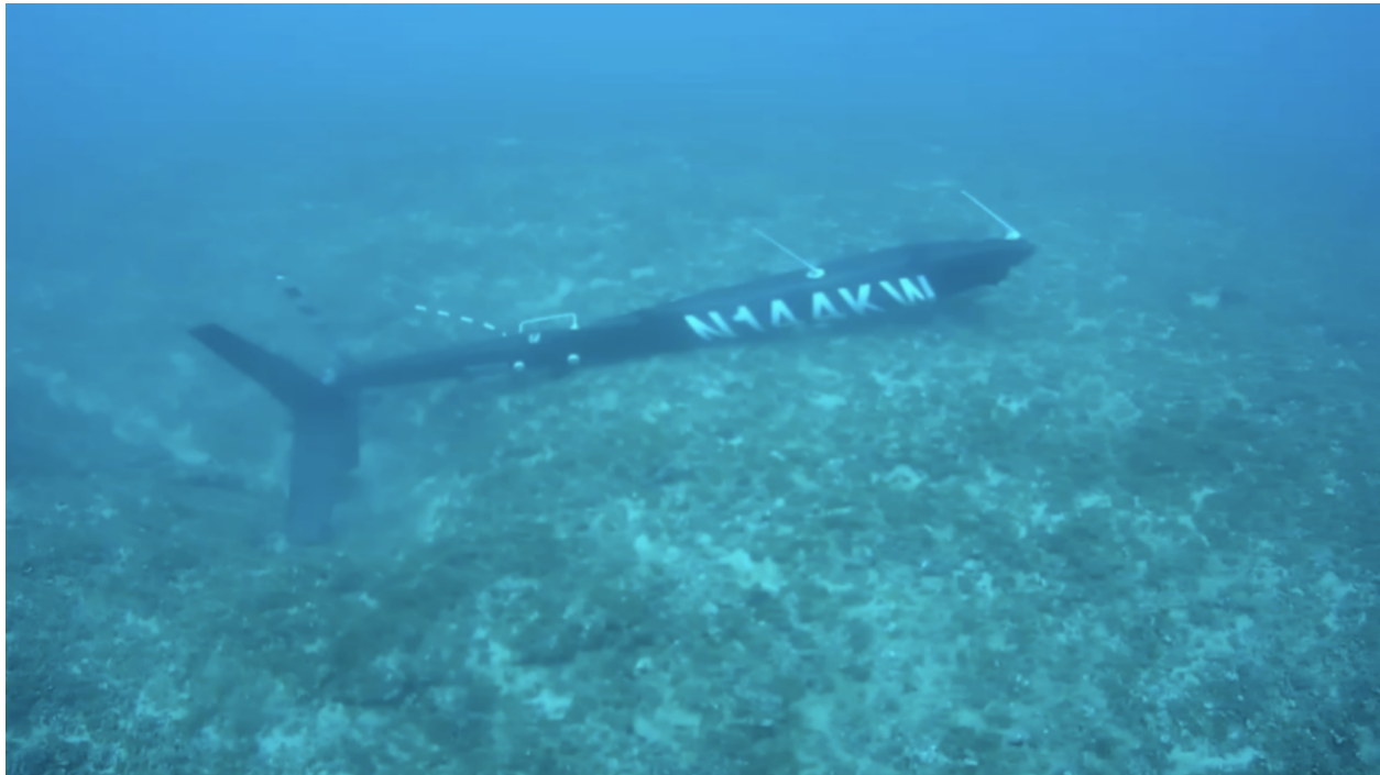
Figure 1. Robinson R44, N144KW, tail boom assembly (US Coast Guard Photo)
