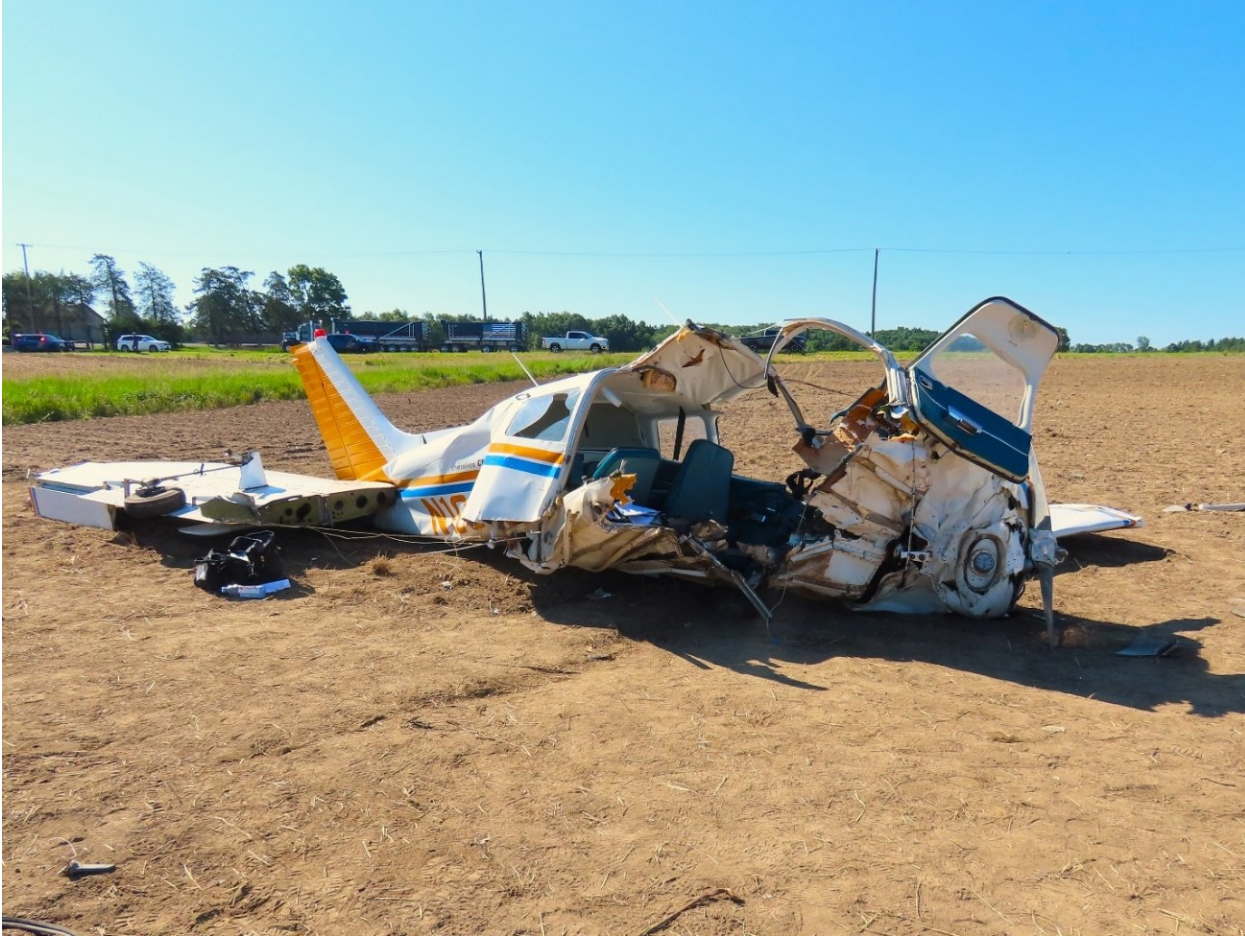
Figure 1. Wreckage with the separated right wing and partially separated forward fuselage.
