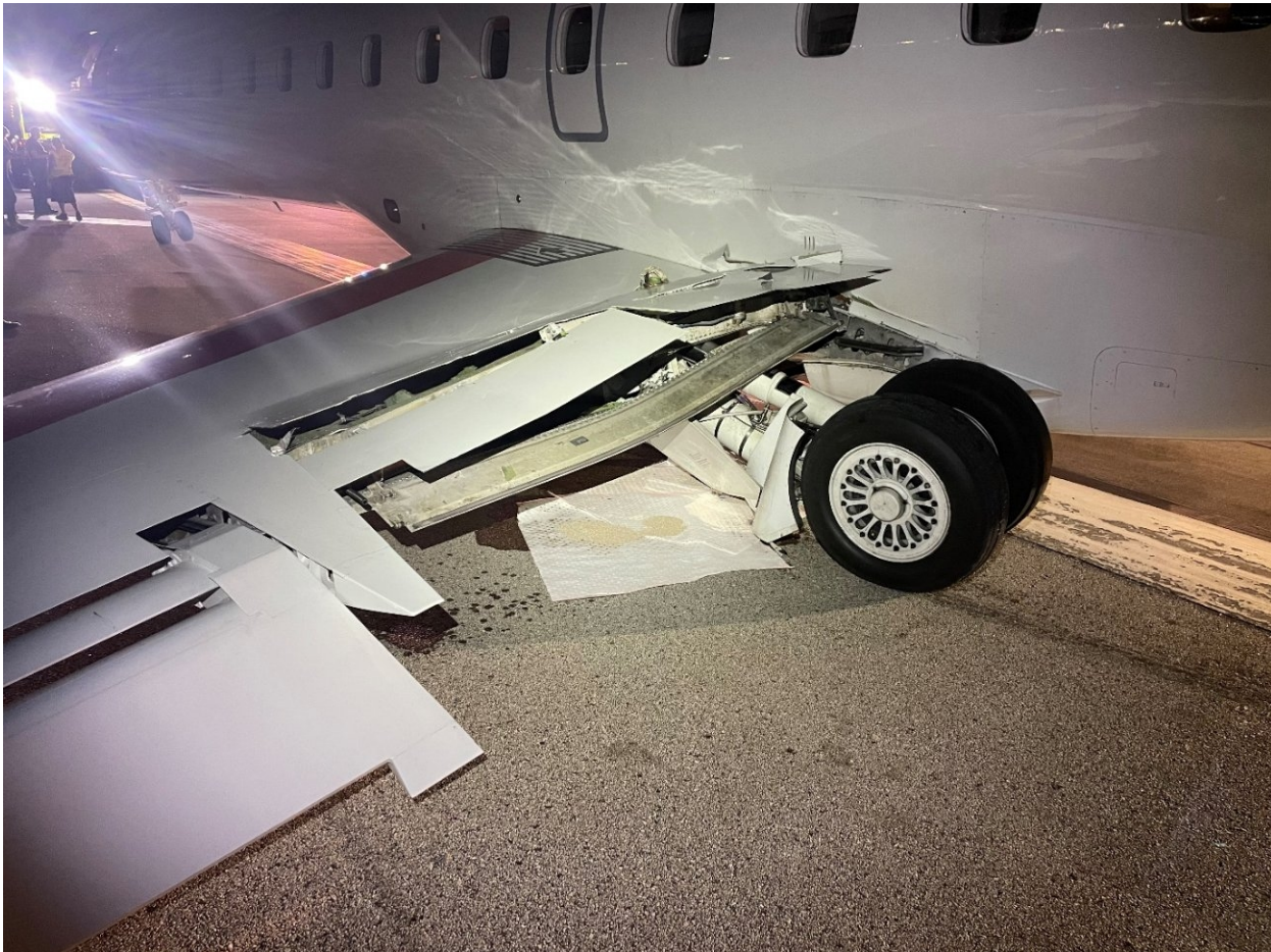
Figure 1. Photograph of the accident aircraft showing the collapsed left landing gear. (Source: FAA)
