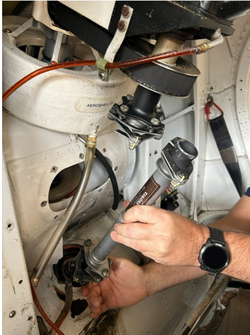
Figure 1: Fractured main rotor drive shaft (Courtesy of FAA)
