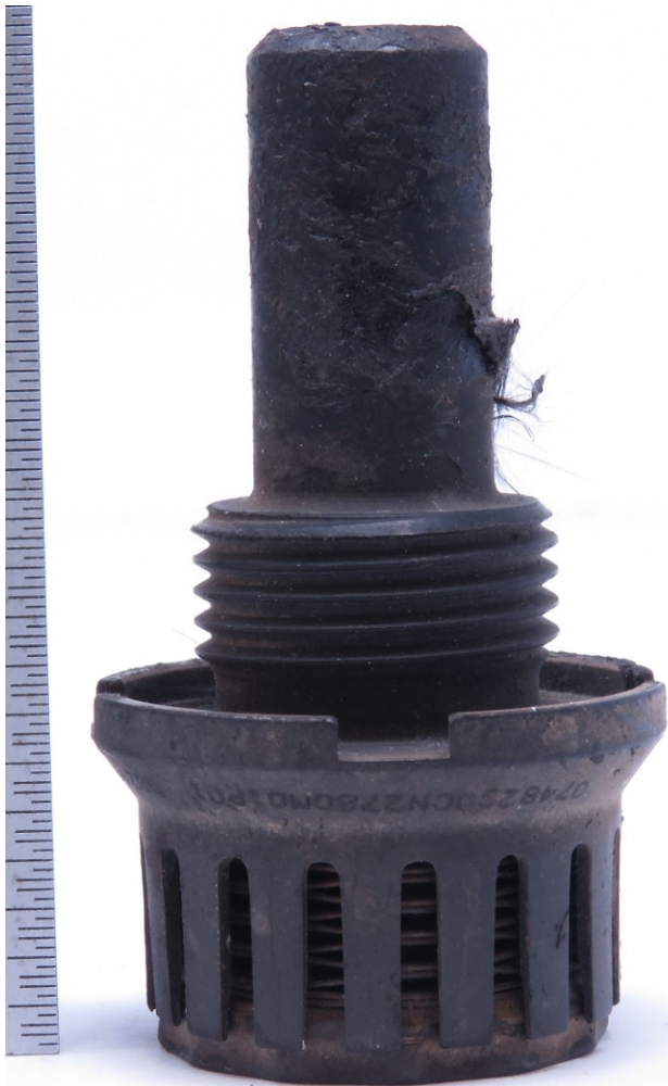
Figure 4. Borescope plug recovered from the incident airplane (Source: General Electric).
