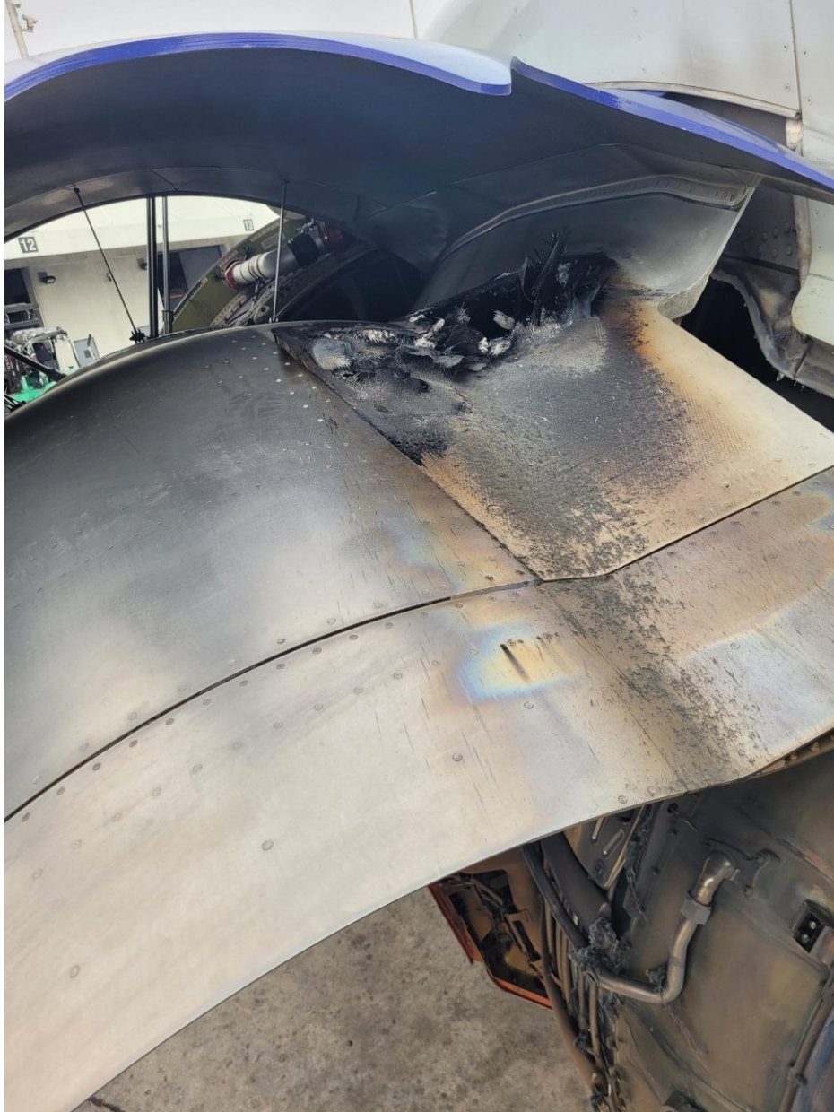
Figure 3. Burned area above borescope port M (Source: Atlas Air).
