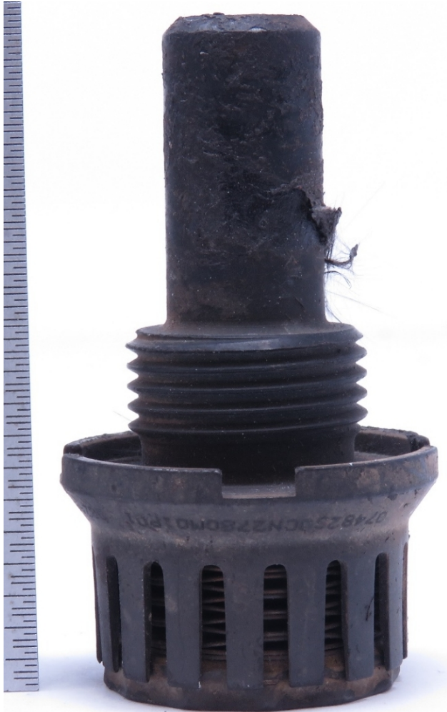
Figure 4. Borescope plug recovered from the incident airplane (Source: General Electric).
