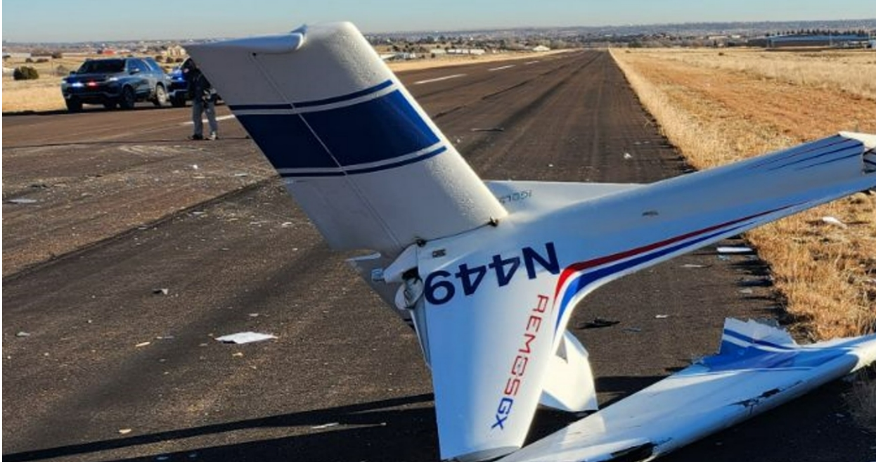
Figure 1-Accident site, aircraft empennage and frost covering the upper surfaces of the horizontal stabilizer. (Courtesy of the Airport Manager)
