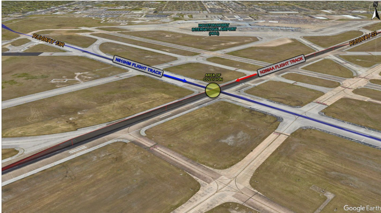
Figure 1. View of both airplanes flight tracks with the area the ground collision occurred highlighted in yellow. The blue line represents N510HM, and the red line represents N269AA.
