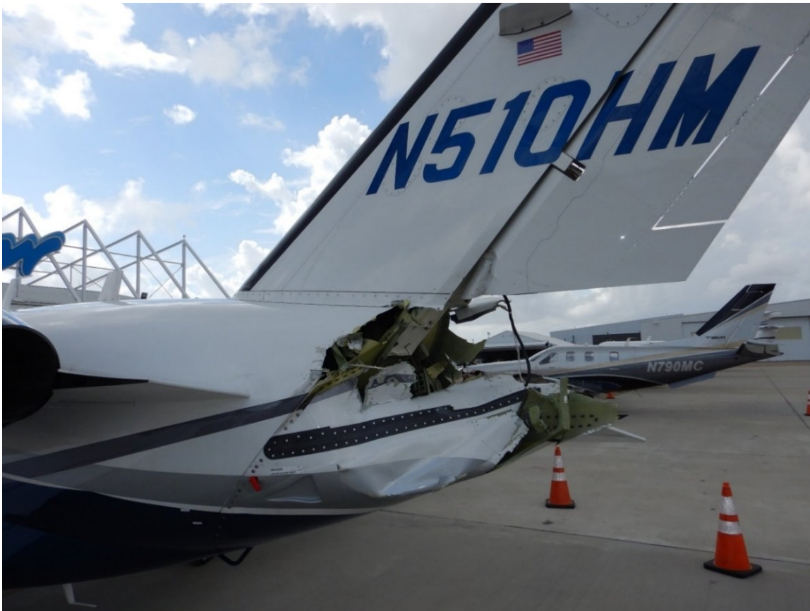
Figure 4. Left side view of N510HM's damage to its empennage.
