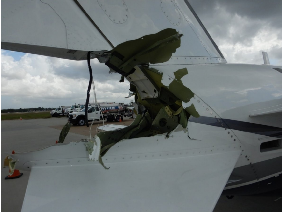
Figure 6. Right side view of N510HM's damage to its empennage.
