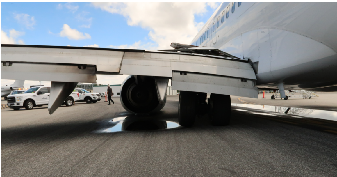
Figure 1. Photograph showing collapsed left MLG and engine resting on the ground.
