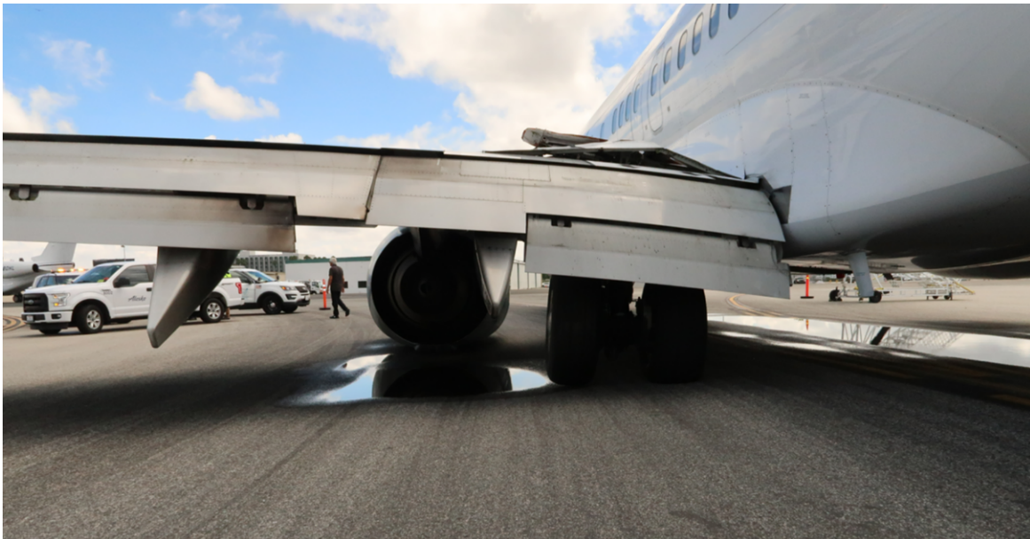
Figure 1. Collapsed left MLG and engine resting on the ground.
