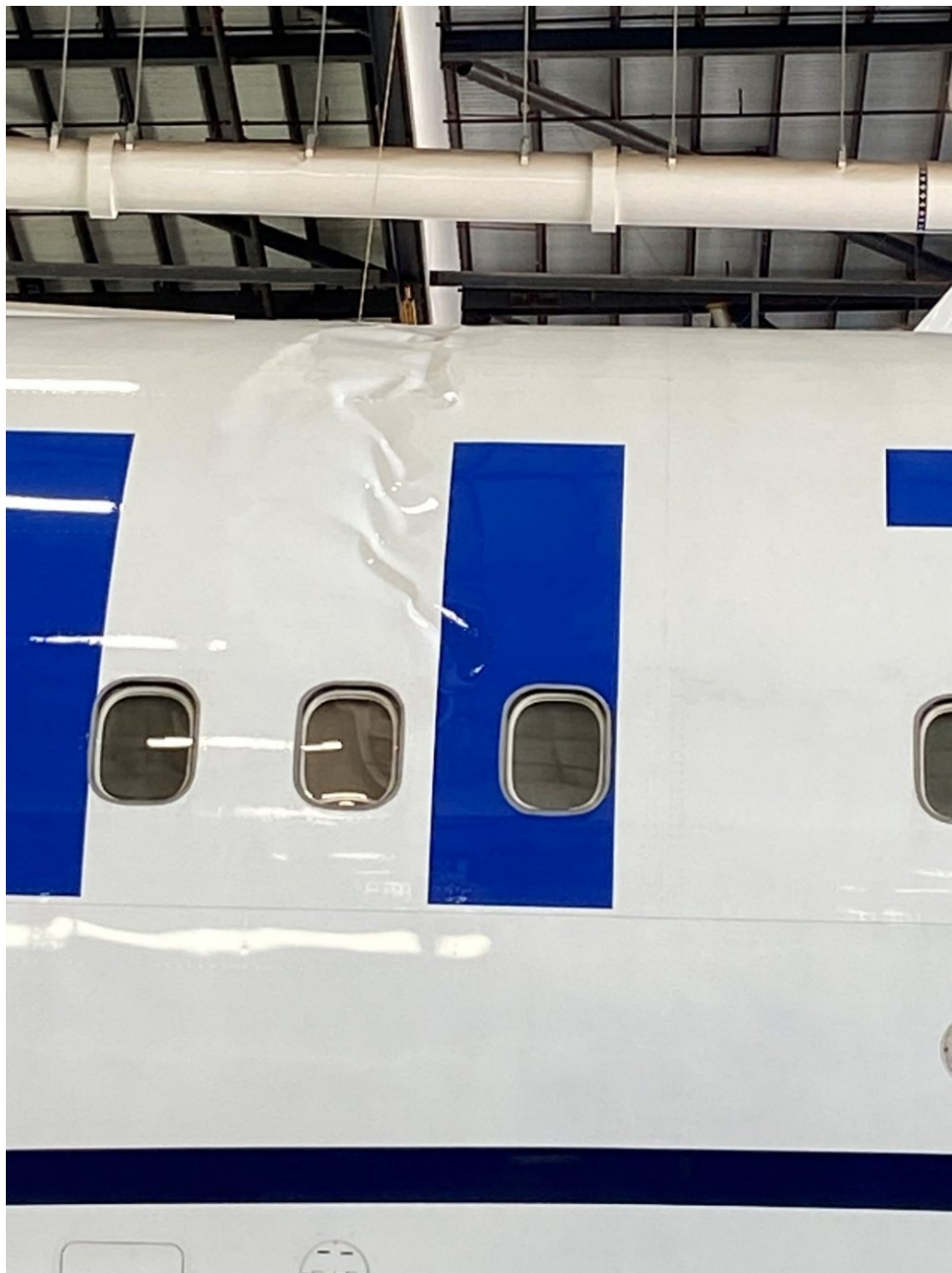
Figure 1. Close up view of damage to the airplane (source: United Airlines).
