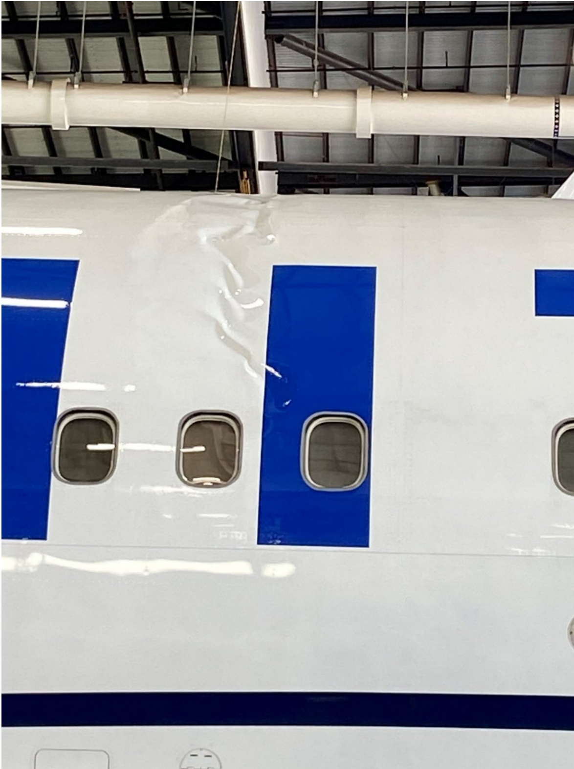
Figure 1. Close-up view of the airplane damage on the left side of the fuselage (Source: United Airlines).
