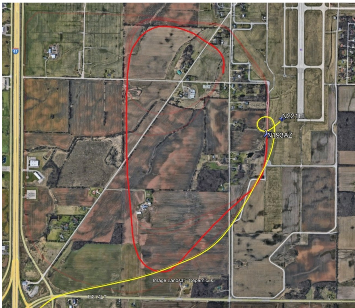
Figure 1. Flight tracks of the helicopter (red) and gyroplane (yellow).
