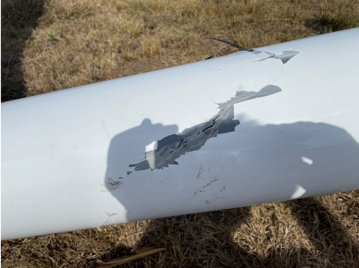
Figure 1. Tail boom structure cracks
