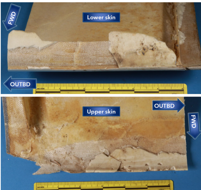
Figure 4. Sectioned right wing lower skin (upper image) and upper skin (lower image) after the upper skin was separated from the spar. The lower skin shows mating fracture surfaces at the inboard end of the leading-edge bond line.
