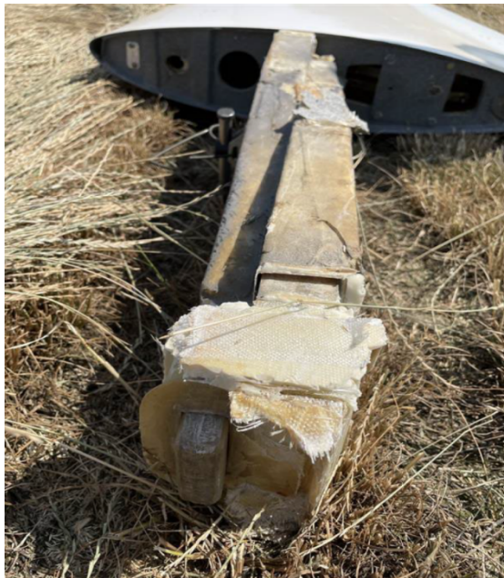
Figure 1. Accident site image of right-wing spar fracture separation.
