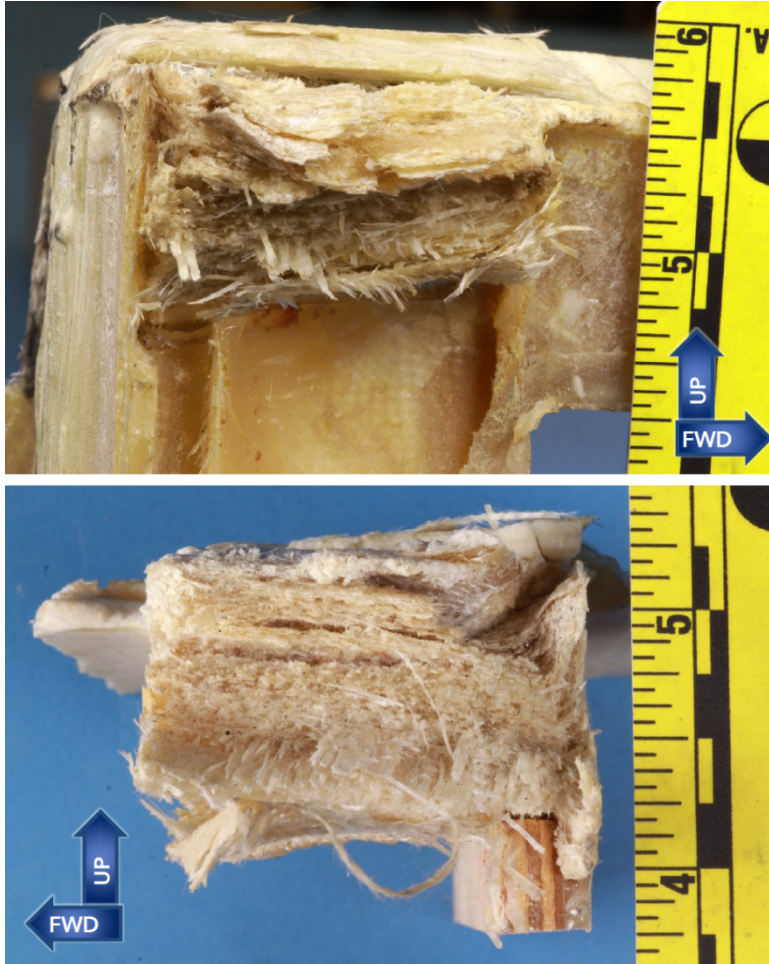
Figure 6. Inboard side (upper image) and outboard side (lower image) of the right-wing spar upper cap fracture.
