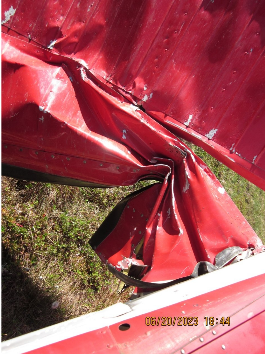
Figure 3 View of the aft crushing on the horizontal stabilizer.
