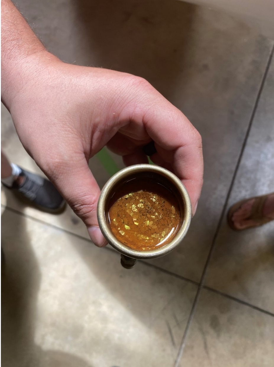
Figure 1. – View of gascolator with rusted particles, water, and trace amounts of fuel as found (source FAA).
