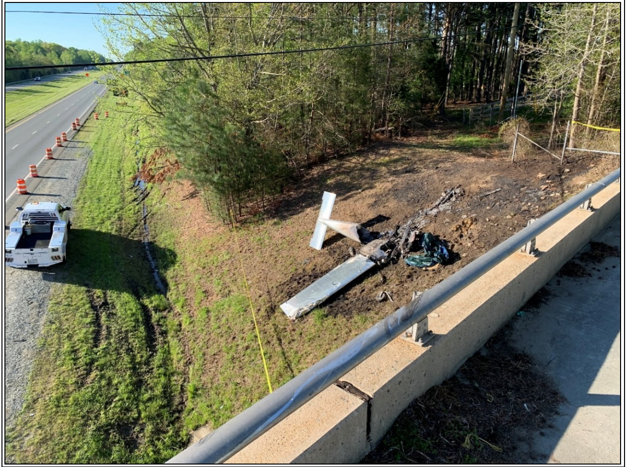
Figure 3 - Overview of the accident site as viewed from the overpass the airplane impacted. Note the powerlines above the overpass, which spanned across the entire highway from east to west.
