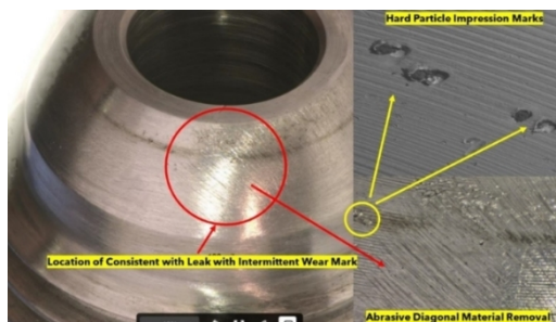
PHOTO 3: No. 18 FN MALE BULLNOSE WITH ABRASIVE MARKS AND PARTICLE IMPRESSION
