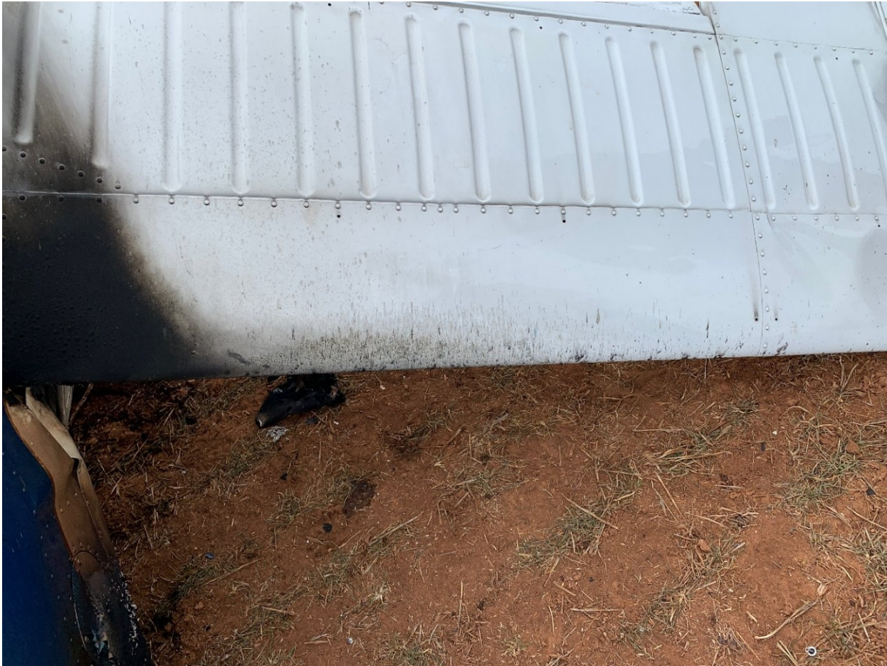
Figure 4. Oil streaking on the underside of the left horizontal stabilator.
