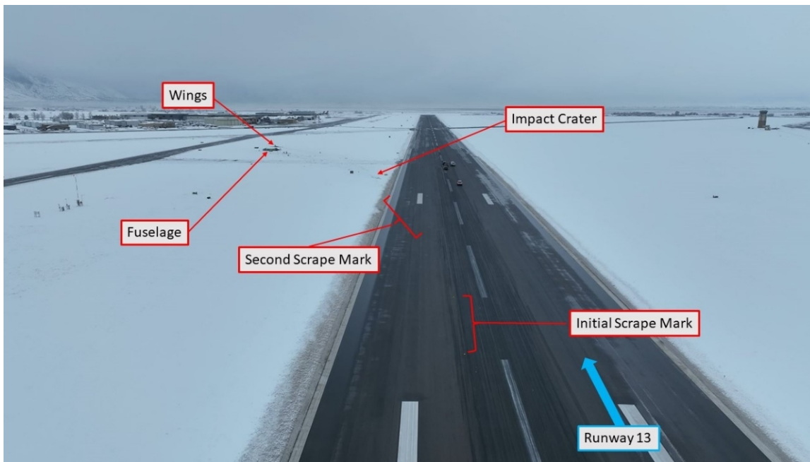
Figure 1: Aerial overview of the accident site. Image courtesy of Provo Police Department with NTSB annotations.
