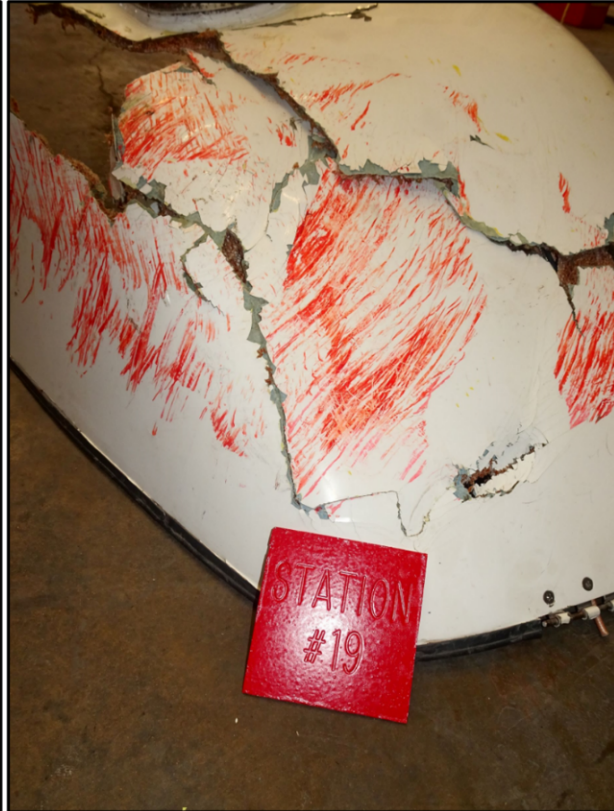
Image 3a (left) – Damaged perimeter light from west edge of helipad Image 3b (right) – Upper hydraulic servo cover with red paint transfer and exemplar paint sample from platform.
