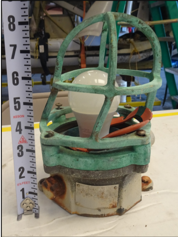
Image 3a (left) – Damaged perimeter light from west edge of helipad Image 3b (right) – Upper hydraulic servo cover with red paint transfer and exemplar paint sample from platform.
