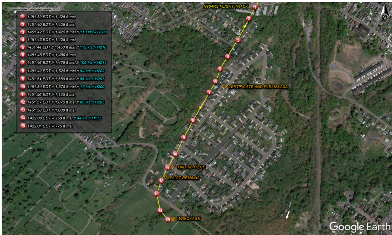
Figure 1 - Flight path (yellow line) with annotated position, time, altitude, ground speed, and path heading. The locations of recovered debris are also plotted.
