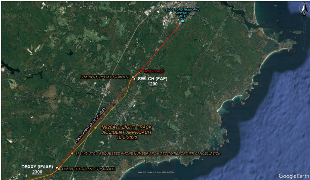
Figure 2 - View of Approach Track of Accident Flight with Altitudes at IAF and FAF (NTSB)
