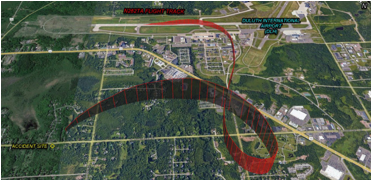
Figure 1 - ADS-B data depicting an orthogonal plot of the airplane's flight track in profile in red.
