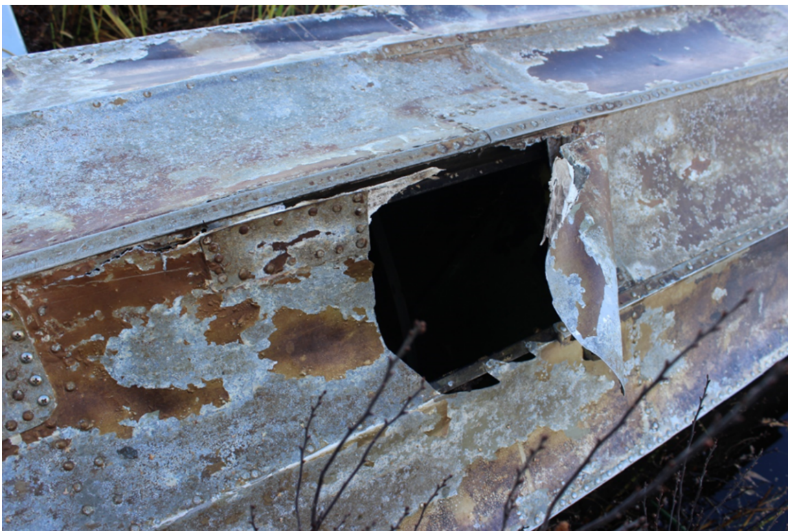
Figure 1 View of partially separated section on hull of the right float.
