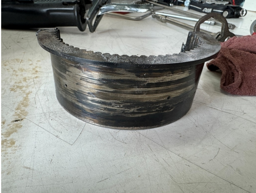
Figure 3: Portion of the front secondary counterbalance bearing.
