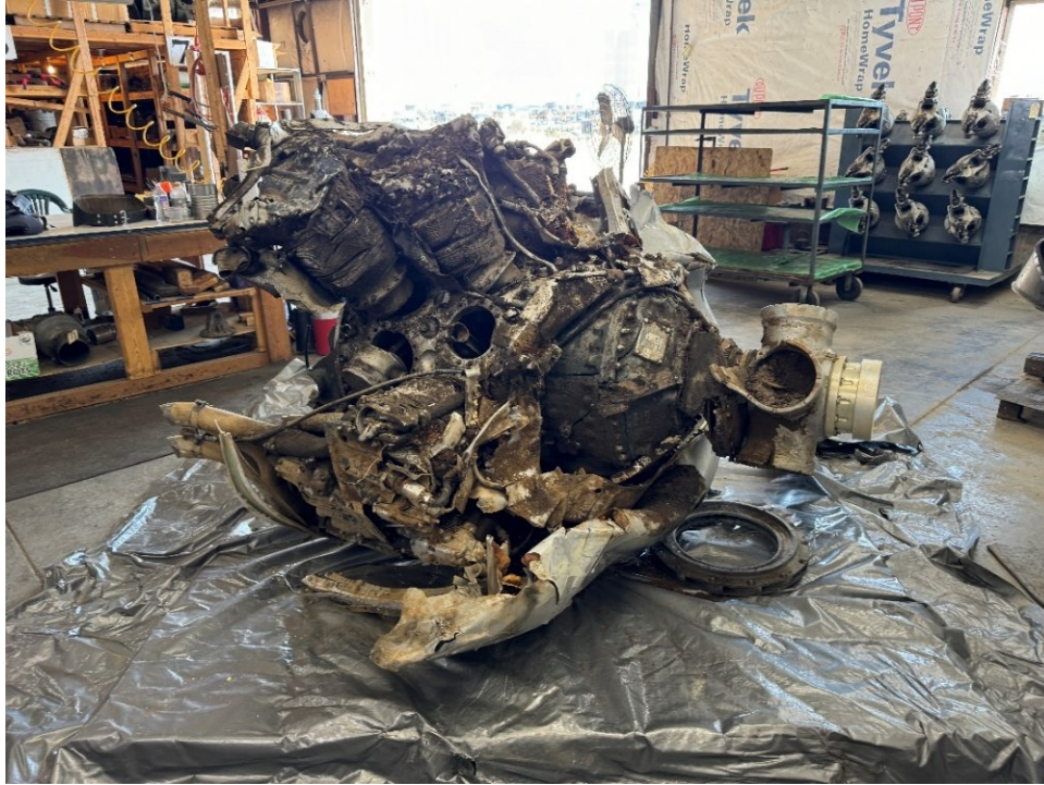
Figure 2: Forward section of the engine with the area of impact damage and displaced cylinders.
