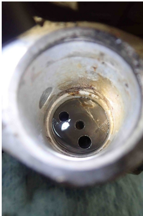
Figure 4 - Corrosion on the surfaces of the idle and mixture valve housing bore
