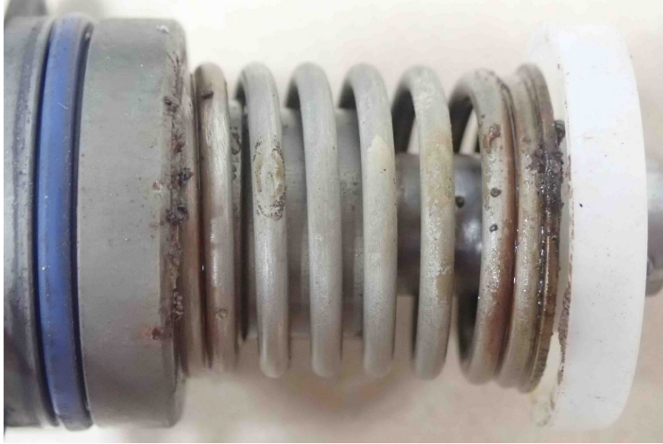
Figure 3 - Corrosion deposits on the lower side of the mixture control spring
