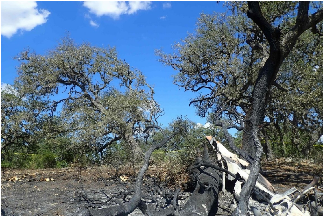
Figure 3 – Facing north, a 60° swath of cut tree limbs and branches, with the main wreckage in the foreground.
