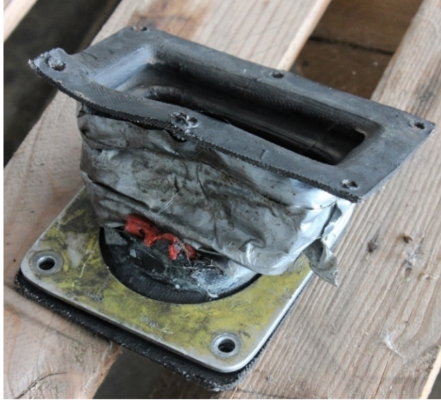
Figure 1. Induction coupling with gray tape.
