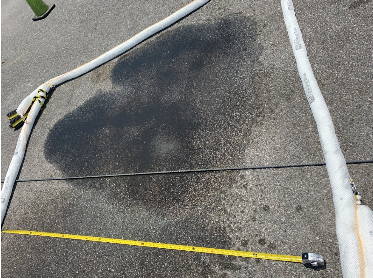
Figure 2 - Large oil stain on the pavement where airplane was located at engine start.
