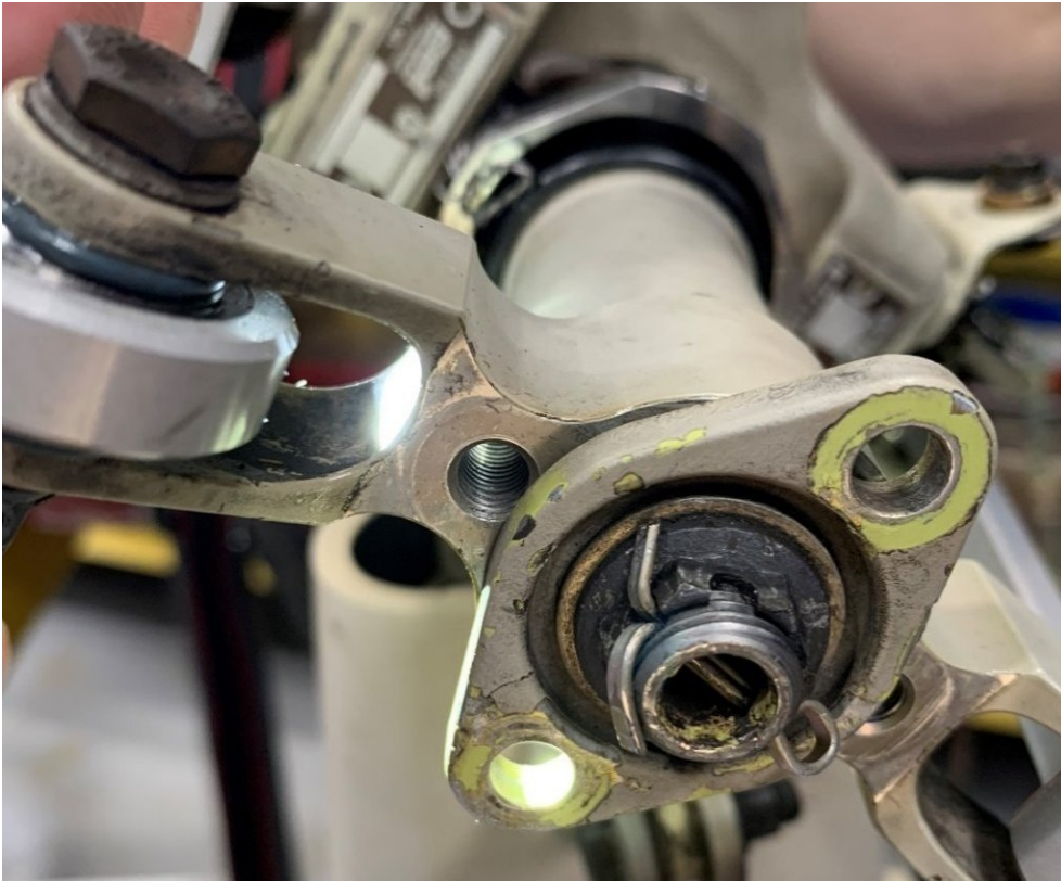
Figure 2. Tail rotor crosshead/drive plate attachment bolt bore threads (Source: Bell Helicopters).
