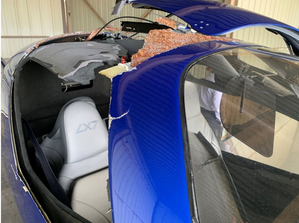
Figure 1- View of missing right front window and roof structure. (Photo courtesy of FAA)
