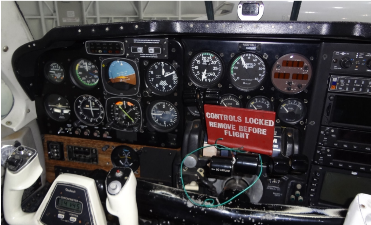
Figure 2. Instrument panel similar to accident airplane (Note: dual yoke was not installed on the accident airplane)
