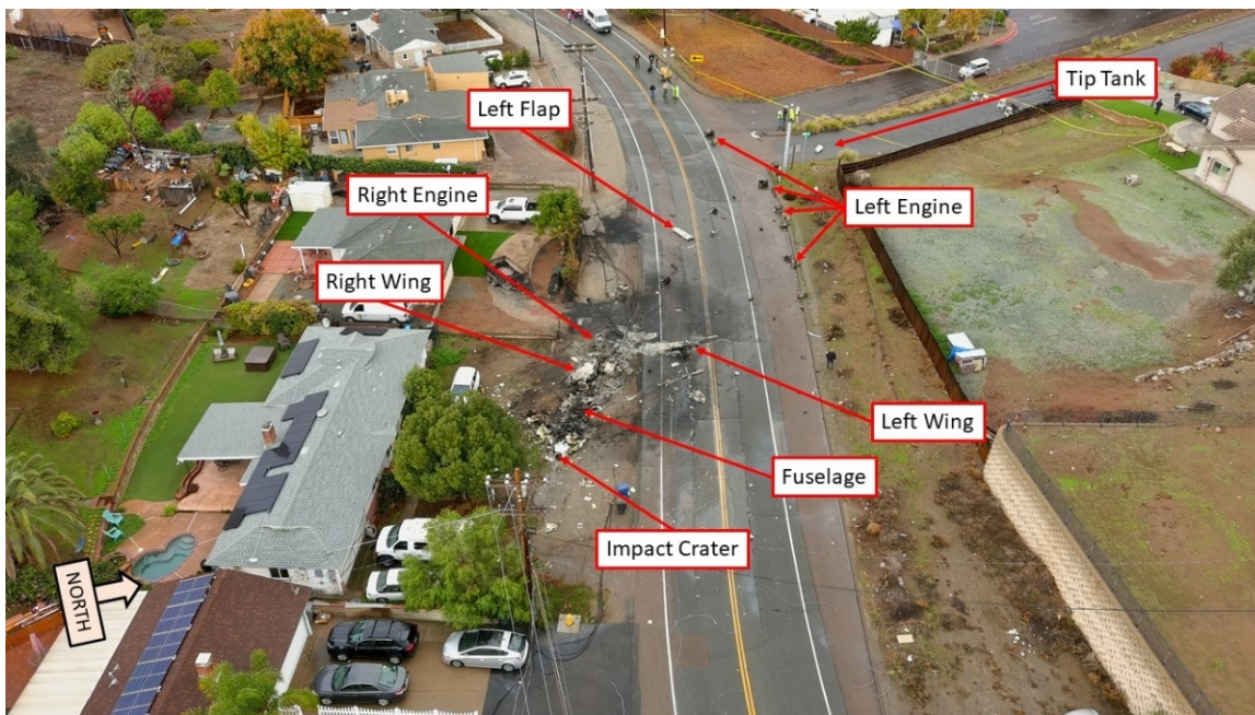
Figure 3: Accident site aerial photo (Courtesy of the San Diego Sheriff Office) with NTSB annotations.
