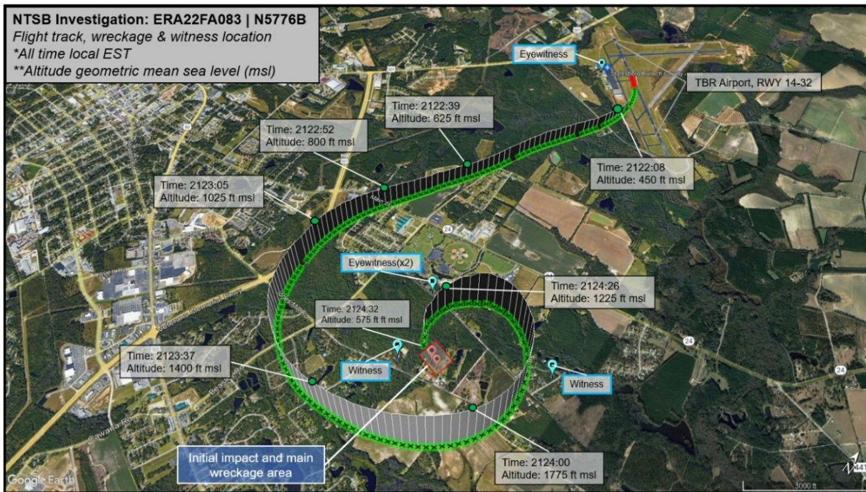
Figure 1: Overview of the flight track, wreckage, and witness locations.
