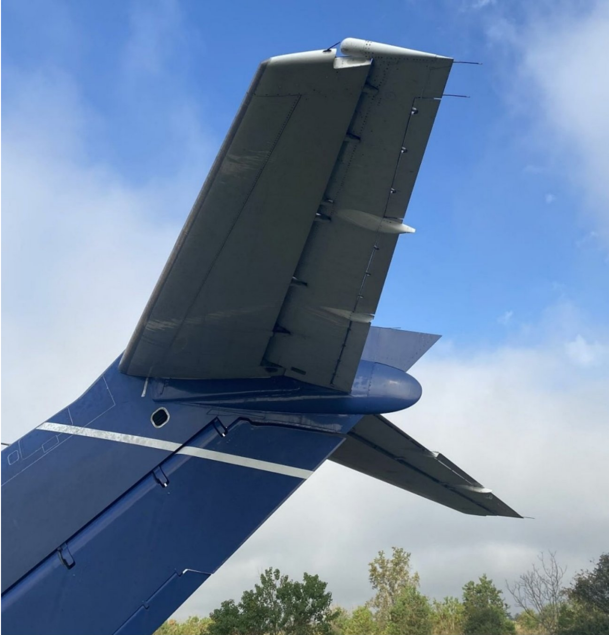
Figure 4. Both elevators as found in the trailing-edge down position.
