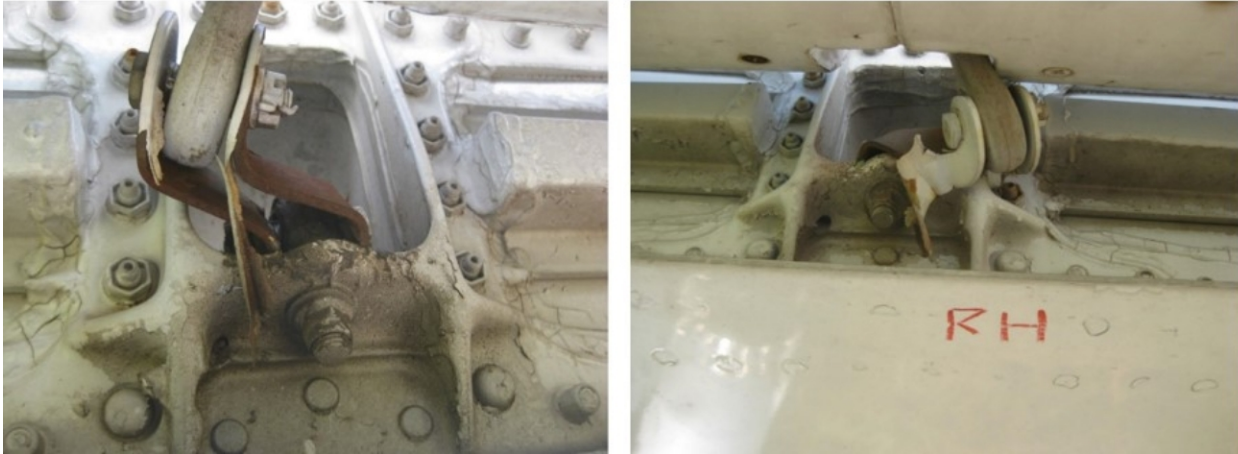
Figure 5. Left and right elevator inboard geared tab linkages (left and right, respectively), viewed from underneath each elevator. Each linkage is bent outboard.
