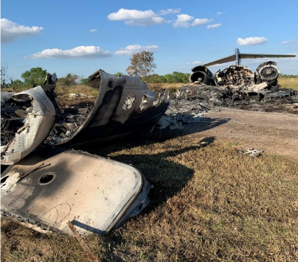
Figure 3. View of the wreckage (from front left looking aft) showing heavy fire damage forward of the empennage.
