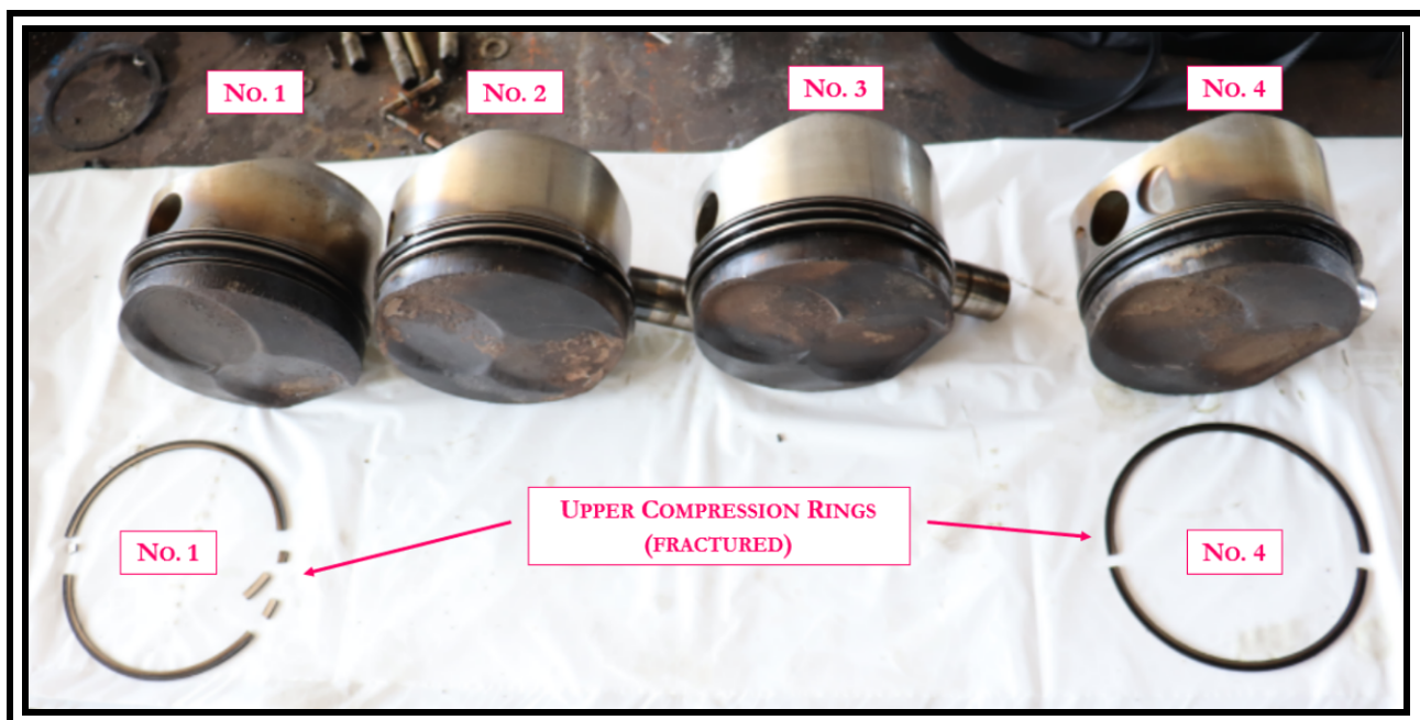
Figure 5: Fractured rings from the Nos. 1 and 4 pistons.
