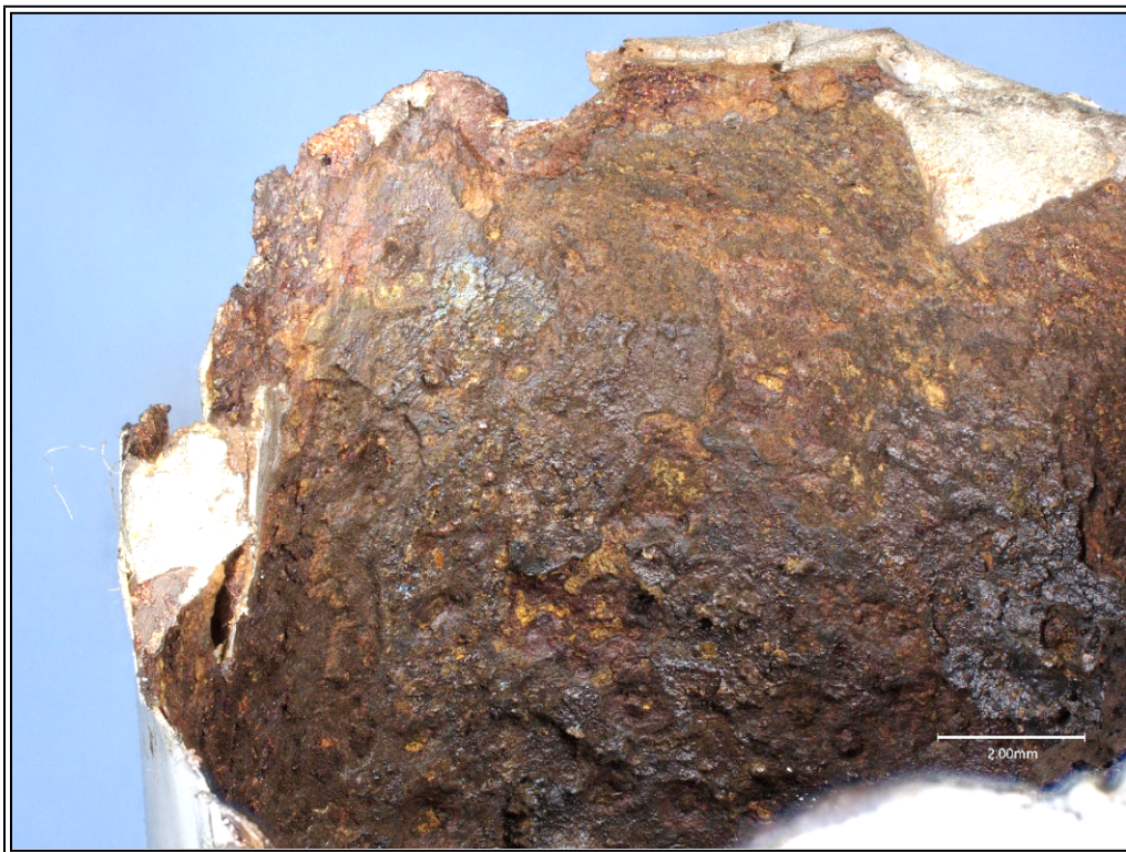
Figure 7. Inner surface of control tube near the clevis fitting fracture.
