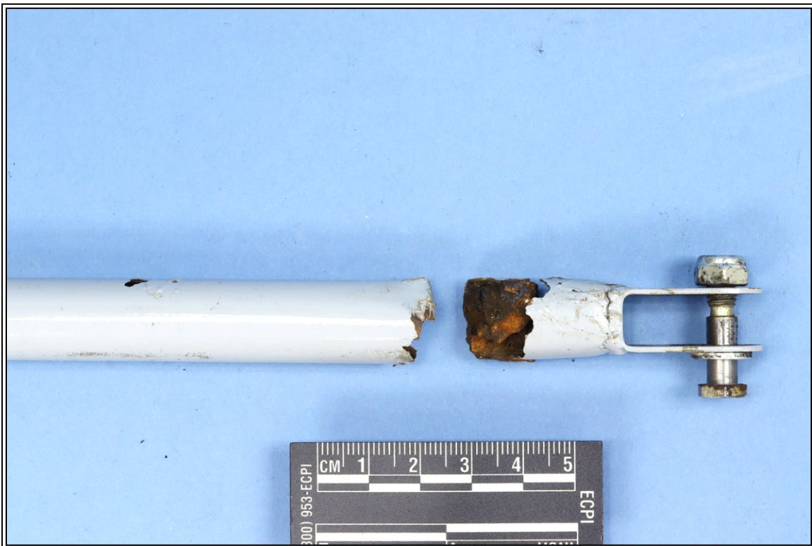
Figure 2. Fracture of elevator control tube near the clevis fitting.
