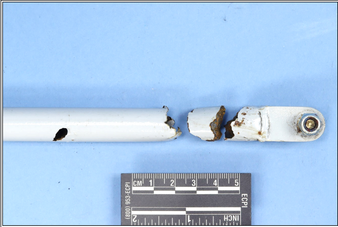
Figure. Fracture of elevator control tube near the clevis fitting.
