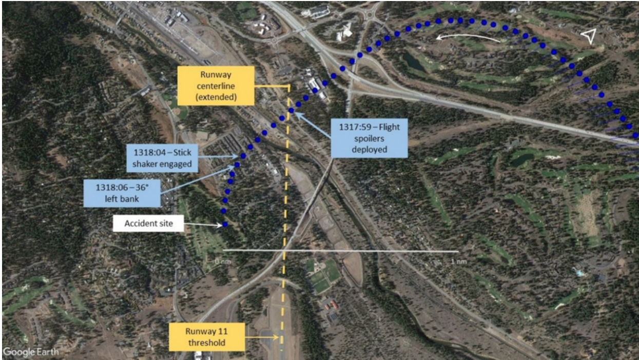
Figure 3. Accident airplane's flightpath during final approach after crossing the runway centerline.
