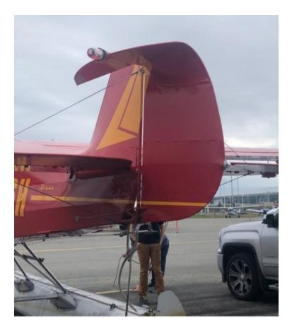
An initial examination of the rudder revealed that the vertical spar tube separated above the upper hinge point and the top portion of the rudder folded over the horizontal stabilizer tail brace wires. (See figure).
