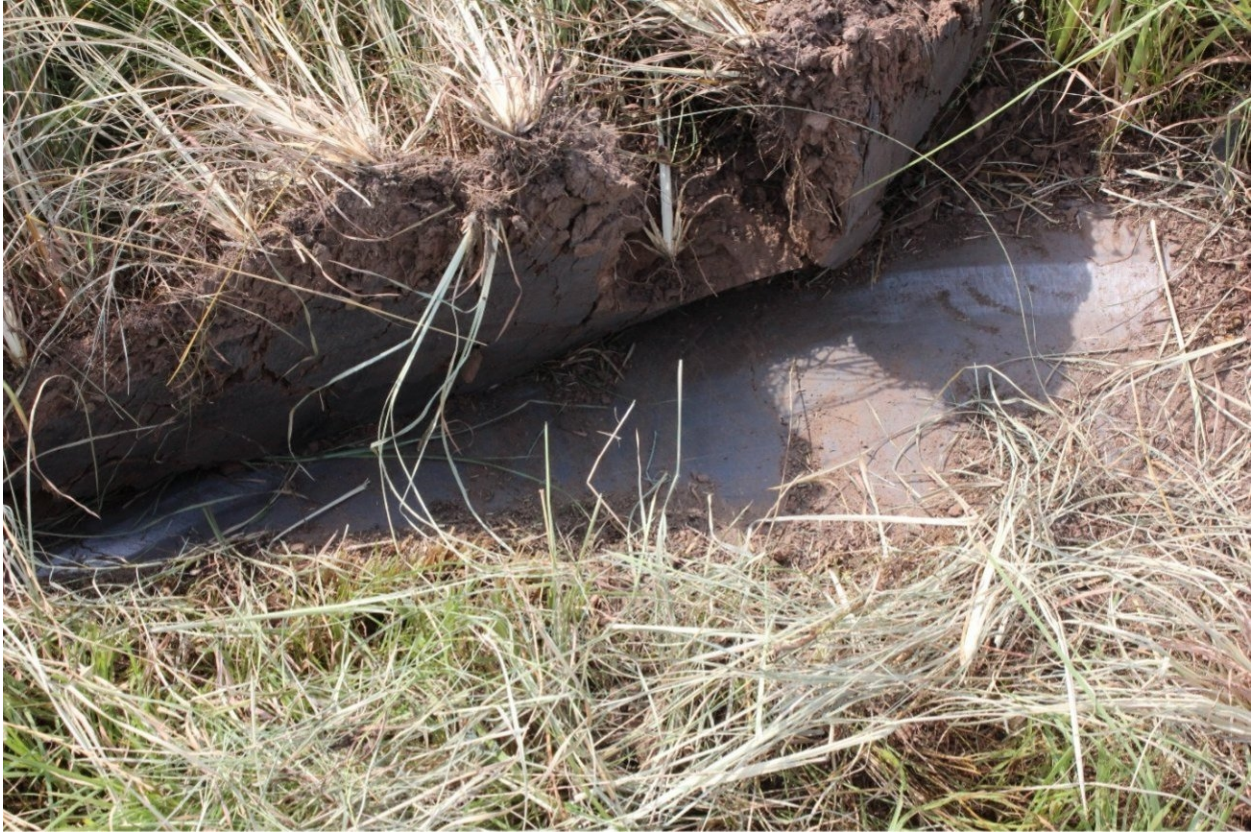
Figure 2: Propeller slash mark with white paint transfer
