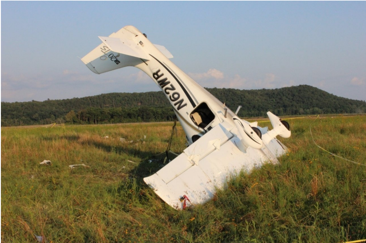
Figure 3: Airplane as it came to rest with pitot tube cover secured in place
