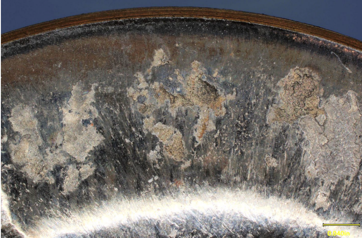
Figure 2. Worn areas of the #2 exhaust tappet head, showing spalling and pitting.
