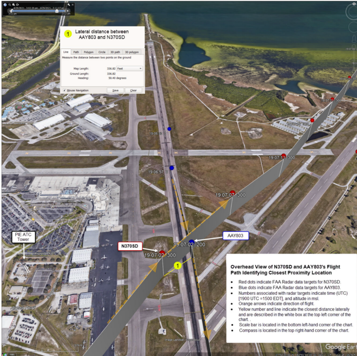
Figure 2. FAA Radar data overlaid on satellite imagery illustrating the flights routes of N370SD and AAY803, and the location of the closest proximity to each other.
