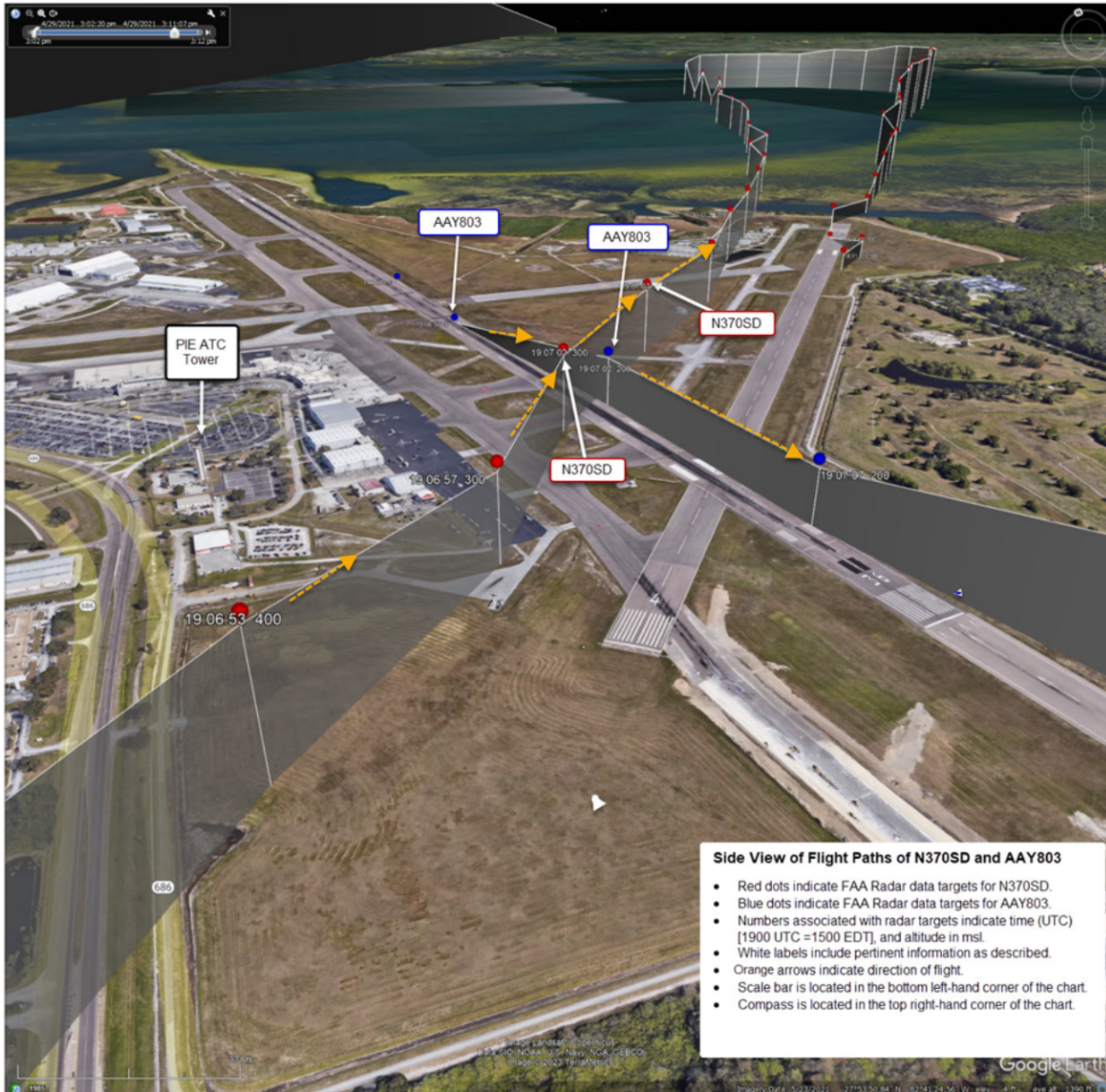
Figure 3. FAA Radar data overlaid satellite imagery illustrating the flight paths of N370SD and AAY803, from a side view perspective.
