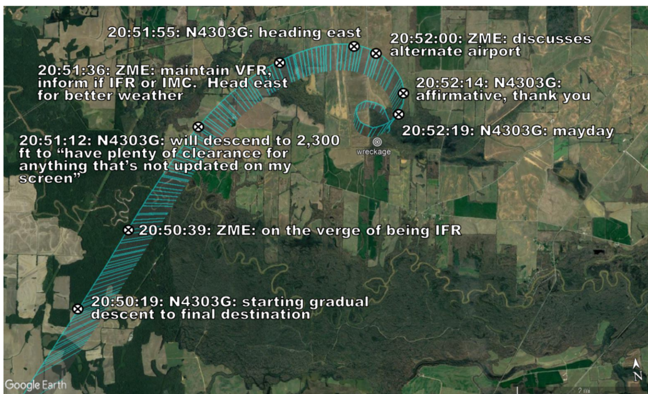
Figure 1. End of flight ADS-B data with controller-pilot communication paraphrased. N4303G is the accident airplane and ‘ZME’ is Memphis Center.
