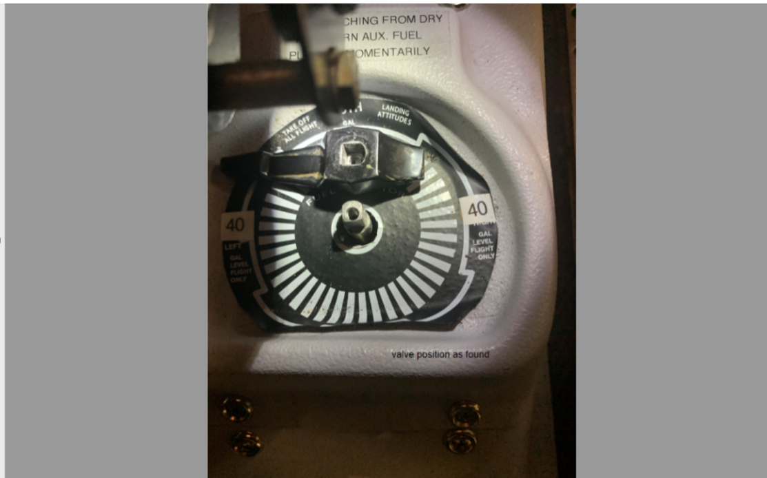
Figure 1: Fuel valve selector (FAA photo)
