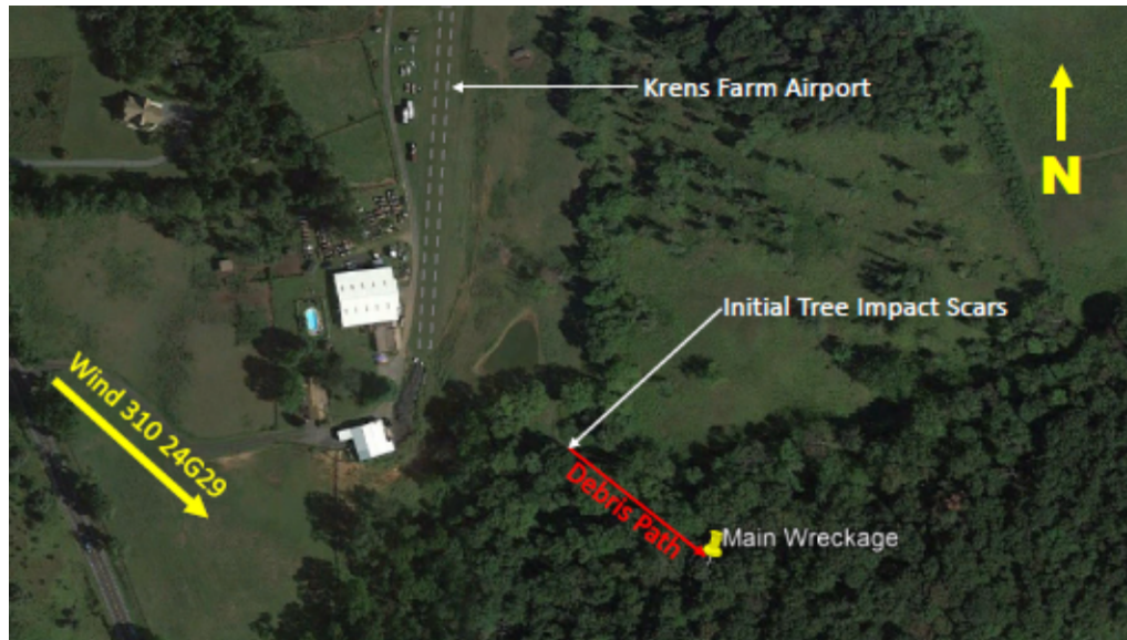
Figure 1 - Accident site diagram depicting runway (dashed white lines), the initial tree impact scars, the debris path, and the main wreckage of the airplane. Also annotated is the reported wind direction and velocity at JYO.
